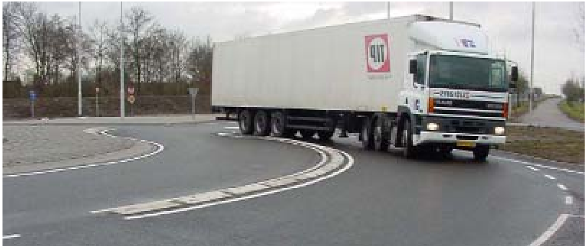
Figure 7: Truck traversing elevated lane divider
